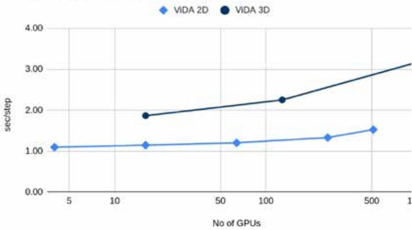
Figure 58: weak scaling of the ViDA code on Leonardo: wall time per single time step as function of number of GPUs . The size of the problem is increased to keep the memory per GPU constant.
