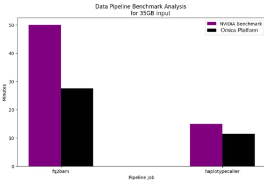
\*Same setup as stated in the Nvidia Parabricks documentation for benchmark purposes (4 NVIDIA V100 GPUs)
