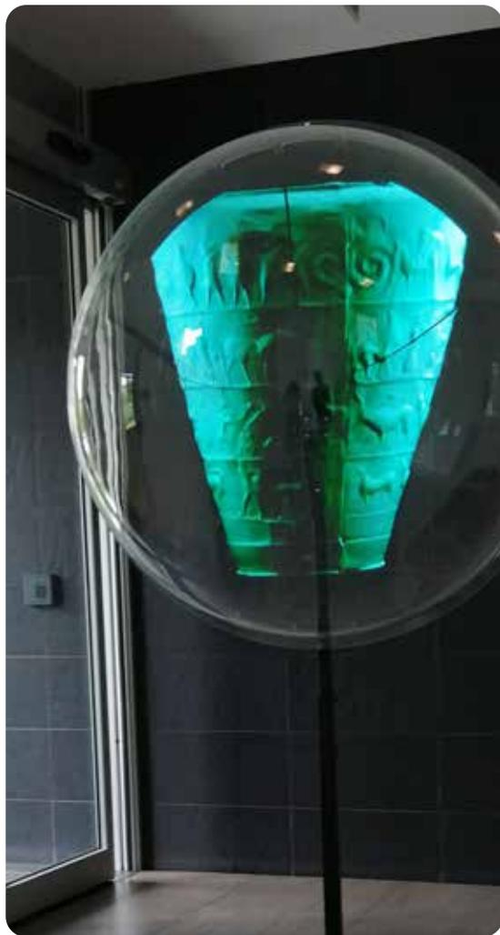
The new portable holographic display, acquired by Cineca, is based on LED technology and is composed of a four-ray rotor display that spins at 670 rpm, creating the optical illusion that shows 3D content floating in midair. The display can show, as a floating hologram, videos or a live stream directly from a computer.
