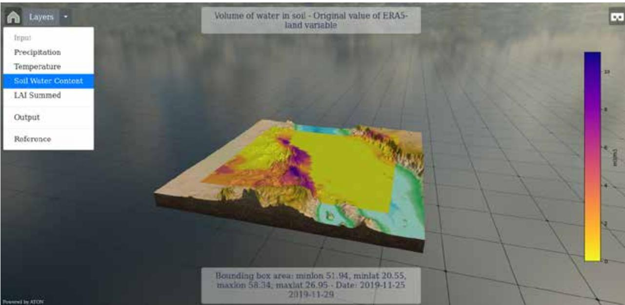
Screenshot of the current state of the Extended Reality (XR) application interface: The requested Earth Observation (EO) data are displayed as selectable layers jointly with a basic set of metadata on the 3D model of the portion of terrain related to their context.
