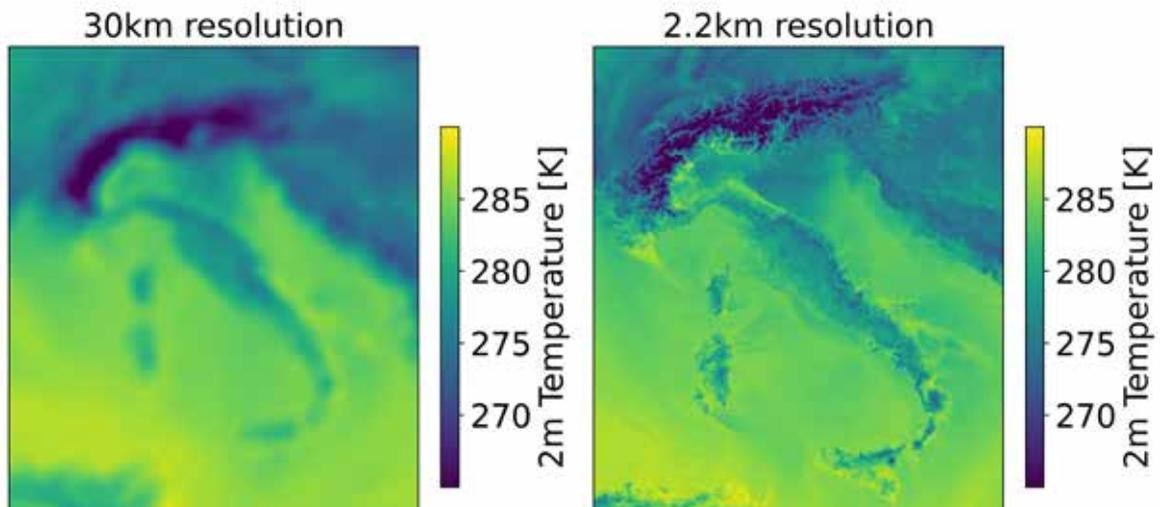
Figure 35: comparison between two maps showing the 2m Temperature of Italy at 30 km and at 2.2 km resolution. The image on the right represents a significant advancement in the accuracy of local phenomena prediction, and it was possible thanks to dynamic downscaling of ERA5.
